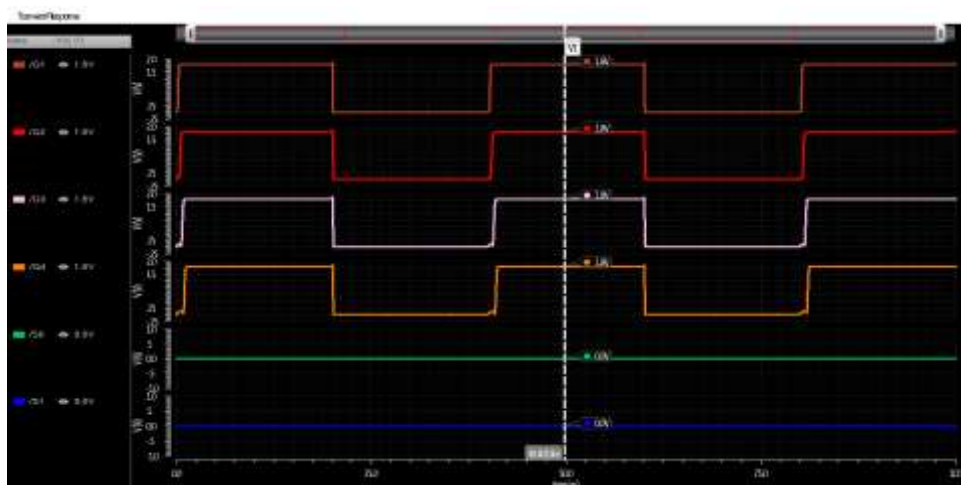
Fig.3(c) Transient response of the proposed 4-bit universal shift registers for parallel load operation
